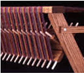
Sectional warp beams have pegs dividing the beam into 1" or 2" sections, permitting the warp to be wound on one section at a time. The warp is wound on from cones or spools on a rack. From the rack the
