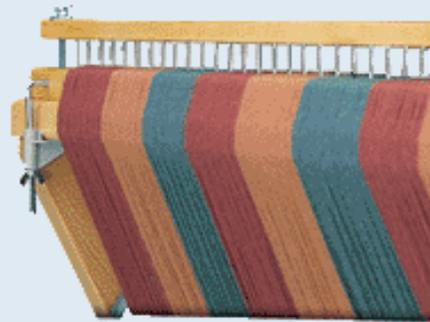
Schacht raddles have built-in clamps for attaching to the back beam. They come with plated pins inserted every inch and with holes drilled every half inch with enough extra pins for half-inch spacing. All Schacht raddles come with tops that are screwed on with wing nuts after the raddle is threaded.
