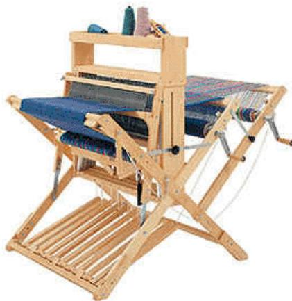
A second beam is useful when you want to have warp threads under different tensions for weave structures such as warp pile and Bedford cord, or when you have a supplementary warp. Predrilled holes in the loom make for easy assembly.
