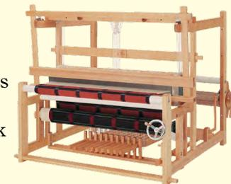
On jack looms, when the treadle is depressed, some shafts raise and the others remain stationary. Jack looms are the most popular style of looms
